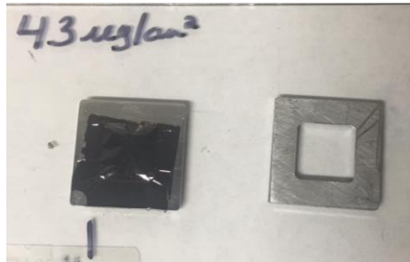
Figure 49: 43 \mu\text{g}/\text{cm}^2 carbon foil floated on frame (left) and bare aluminum frame (right).
